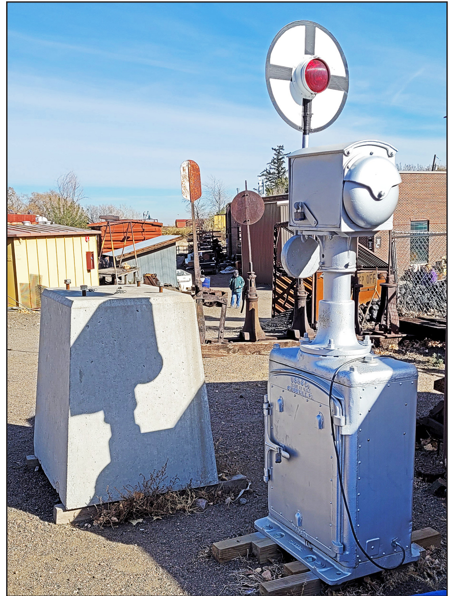
This wig-wag road crossing signal was the last one operating in the state of Colorado. It had been on the old Santa Fe line between La Junta and Trinidad at Delhi until about a year ago. The BNSF retired it, sent it to their signal shop for refurbishment, and then gifted it to the Colorado RR Museum. It should soon be placed on display and in operational condition. Past president Dave Schaaf had a small part in getting it donated to the museum. – Photo © 2022 Dave Schaaf.
